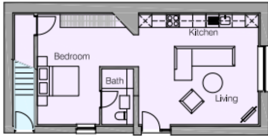
Studio flat 0.1 - Ground 51m 2 gross internal area
